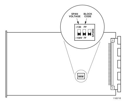
Figure 524-2. RLXIOR Configuration Switches (With Default Settings)
